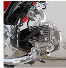
4- Stroke OHV, Cooled by Air
